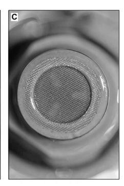
If the control solenoid valve looks like this after cleaning, it needs to be replaced
